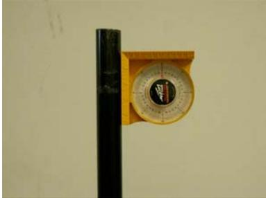
First, makes sure that your pole mount is absolutely vertical. Without vertical pole, all other setting are meaningless.
