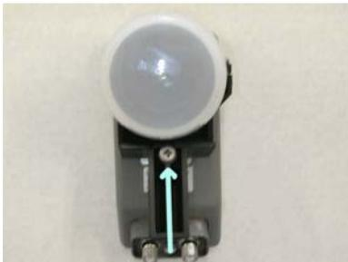
Align the center of **LNB Holder Unit** at the **R10** marking of LNB Guide. Note that each end of the LNB guide has the marking of "L" and "R".
