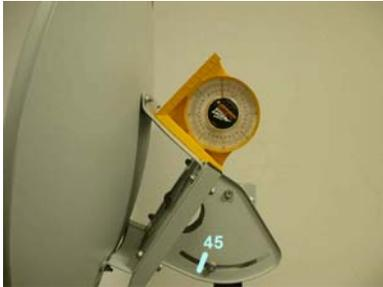
Without any skew adjustment, adjust elevation. You can use an angle locator as shown or use elevation reading on the bracket. (Align the edge of tube to the readings)
