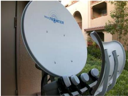
**TIP: Assemble and align Toroidal at ground level** with small TV and receiver right next to you. This will save you a tremendous time. After the alignment, you can put the assembled dish on your roof and adjust azimuth only, take a minute and reducing the risk and sweat!
