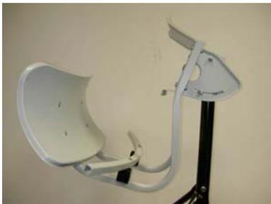
Attach LNBF Guide using B5. Pay attention on the orientation of LNBF Guide. The arc is toward outside from the pole mount.
