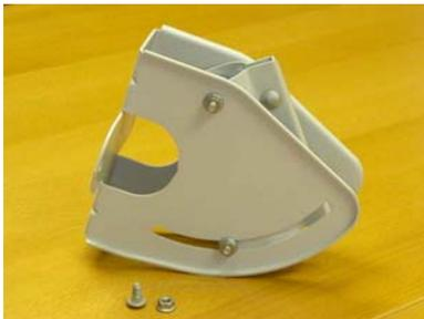
Insert B10, B13. Make sure that nuts are outside of **Back Mount**. This is where you make elevation adjustment later on. For T90, use washer for extra holds. Washer also makes it easier adjusting elevation control later on.
