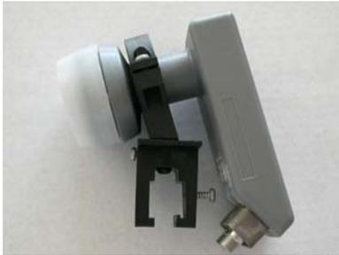
Place LNBF inside the holder and tighten another B6. You may need to **LNB Adapter (A11)** to secure LNBF depending on the neck size of your LNBF.
