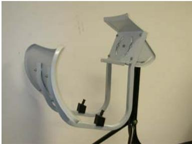
Attach **Sub Reflector** using B2 & B12. You will find a little hold on the center of the side. This side with hole should be placed down.
